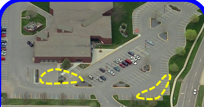
Unused parking was removed to reduce impervious area and provide bioretention cell locations.
